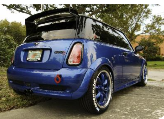
GP-Style wing for non-GP MINI Coopers and custom vortex generators were added to help smooth the airflow over the wing-blade.
