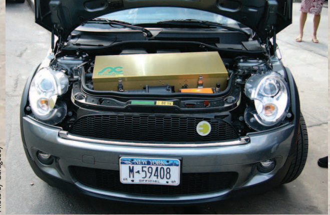
Under the Hood: MINI E's electric motor from AC Propulsion
