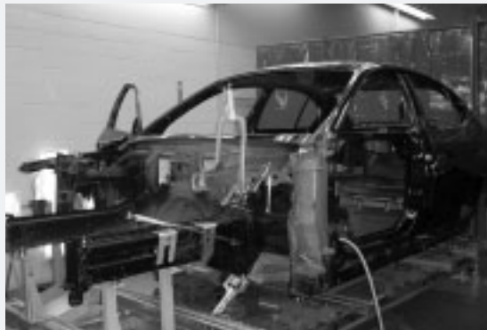
On the Cover: Factory Aluminum Frame Repair Course showing a fully disassembled E60 5-series at the BMW facility in Spartanburg, SC. (photo by Andy Petaludis)
