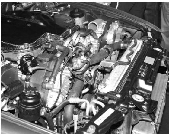
An M5 engine getting a supercharger
