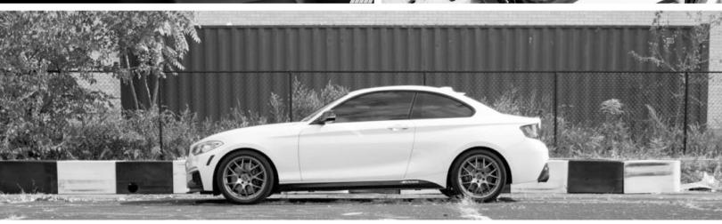
Gunmetal Enkei Tuner Raijin with square 235/40ZR Nitto NT01 DOT-Compliant Competition Road Course Tire. That combined with EBC Yellowstuff pads, MPerformance Rotors, Bimmerworld Insulated F22 Stainless Steel Brake Line Kit, allows him to confidently brake as late as possible and hold some high entry speed in almost stock form.
